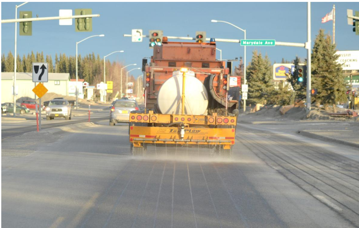
Figure 55 - Soldotna TowPlow Applying Enhanced Anti-Icing Salt Brine
