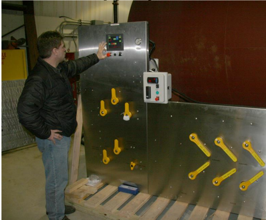
Figure 1 - Salt Brine Control Panel
