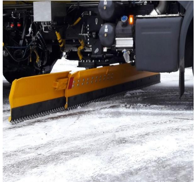
**Underbody plows** go under the body of the truck, between the front and rear axles. Evidently, we are not given to flights of fancy when it comes to naming our plow types! We could have a good competition there!
