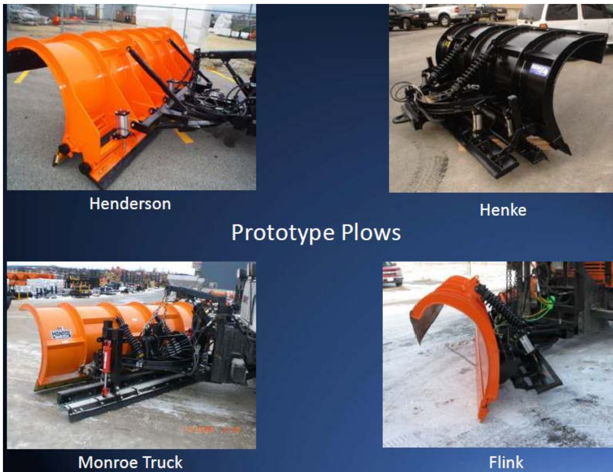
Fig 4. Multi-blade prototype plow designs for the four participating DOTs (courtesy Iowa DOT)
