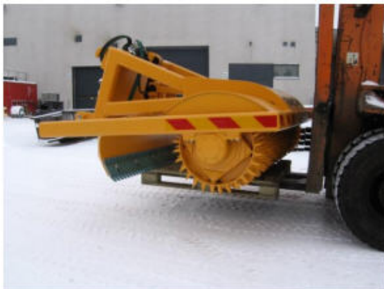
Fig 6. Raiko Wheel Loader Attachment with Plow
