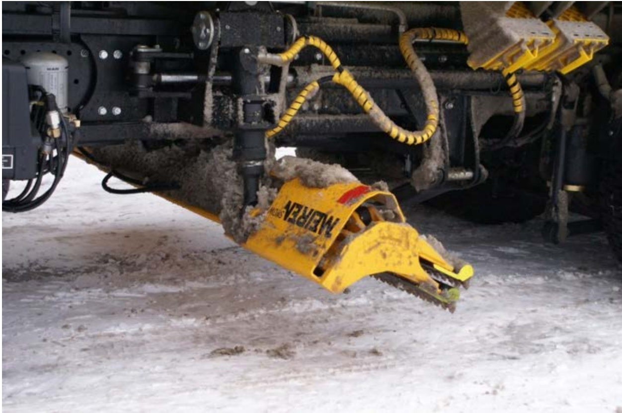
Fig 5. Underbody scraper (courtesy Meiren Engineering)
