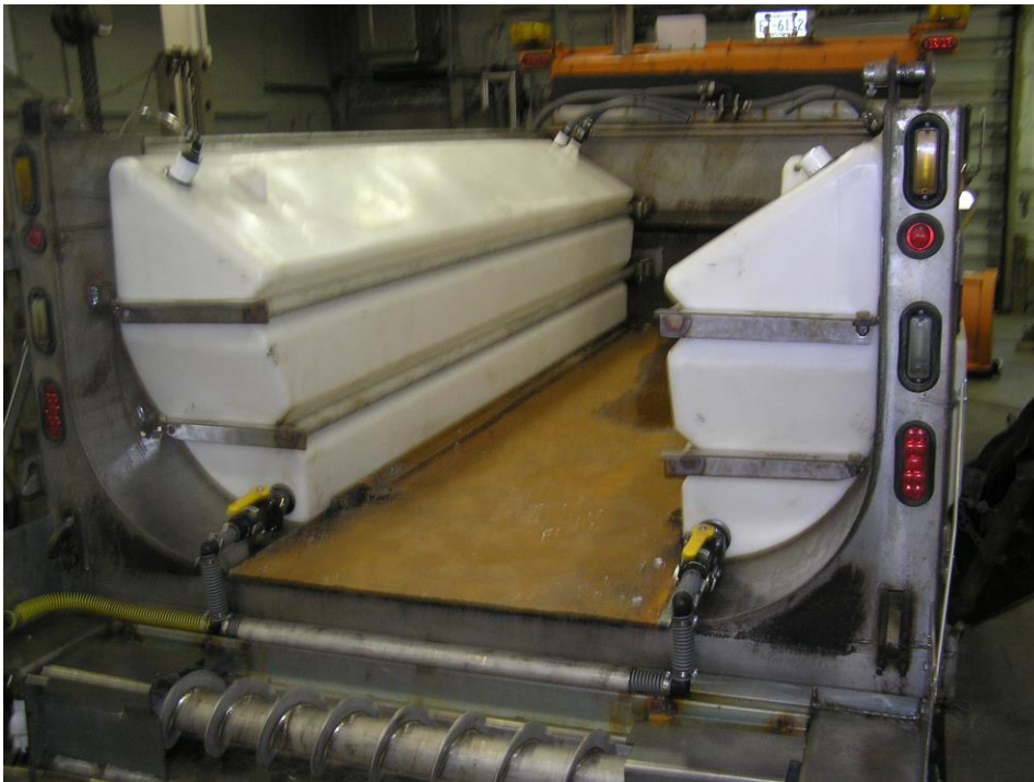
400-gallon tanks for slurry applications
